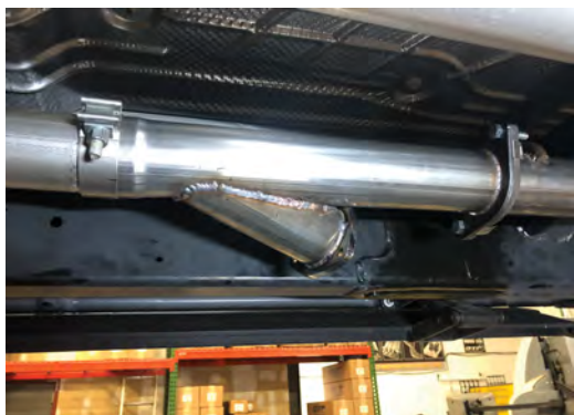
Image B: Aggressor Pipe Installed
