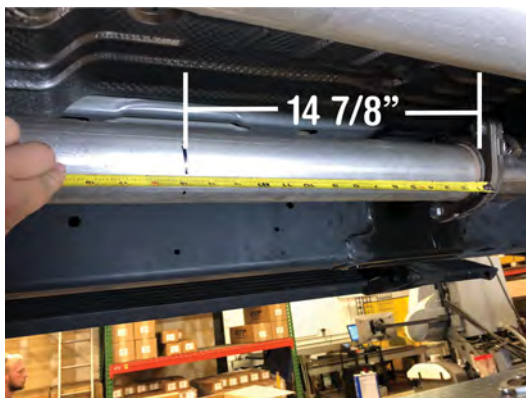
Image A: Cut Location, 14 7/8" from flange
