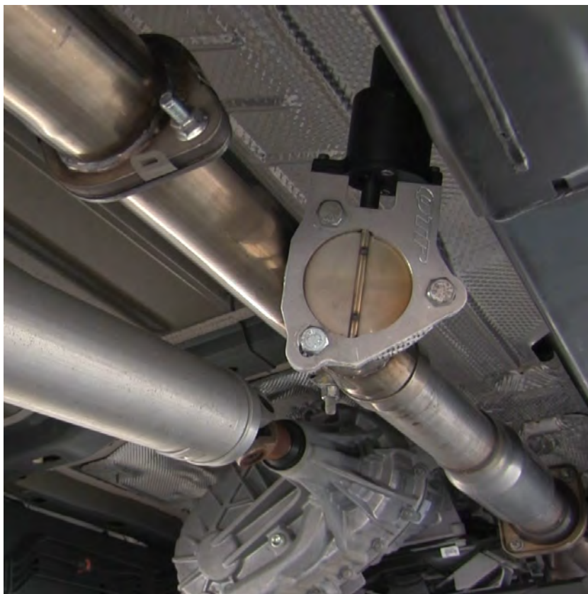
Image C: QTEC Valved installed on Aggressor Pipe
