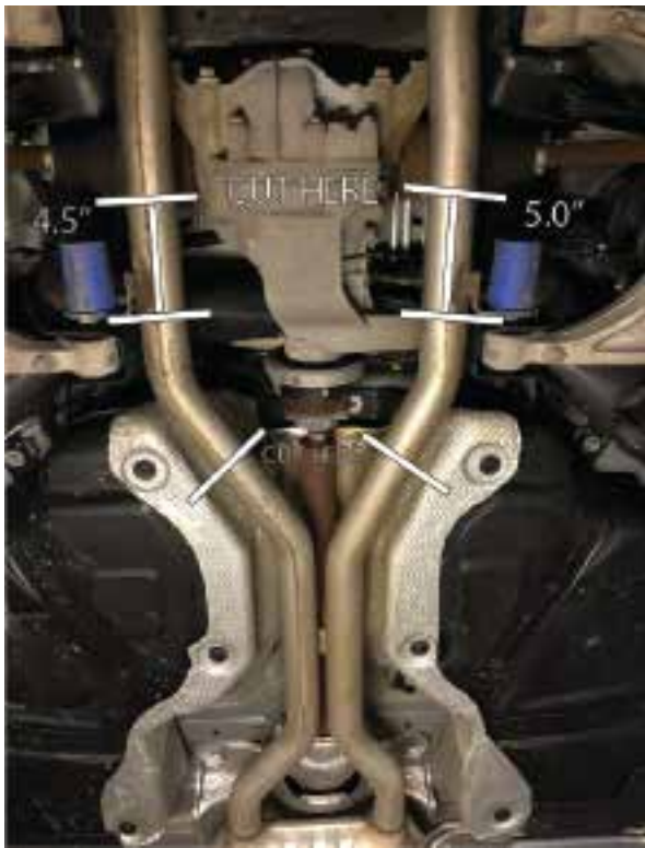
Image A: Cut Locations, measure rear cut, hold up and trace front cut
