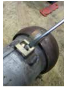
Image B: Pry the lock tang and remove clamp.
