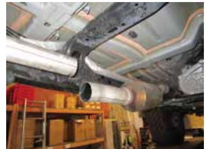
Image C: After the cut remove the resonator and De-Burr the cut.
