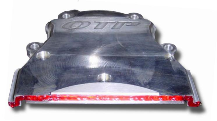
Clean lip area of the top cover. Apply some gasket maker as shown in the picture above. Bolt the top cover to the block. Align both the top and bottom covers so they are even. Torgue bolts to manufactures specs. Bolt back cam position sensor (LS2). Excess sealant can be wiped away with a cloth and shop solvent.
