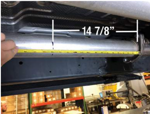
Image A: Cut Location, 14 7/8" from flange
