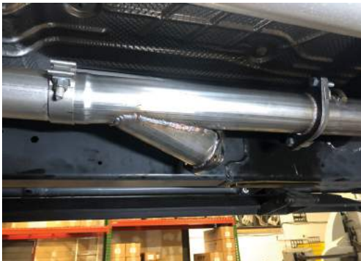
Image B: Aggressor Pipe Installed
