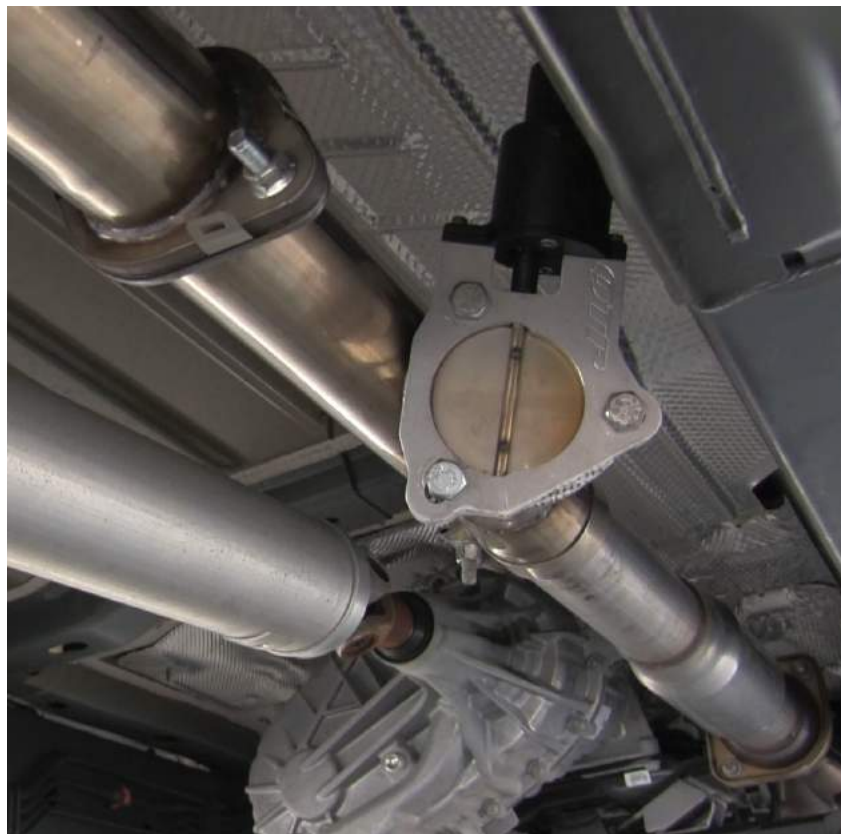
Image C: QTEC Valved installed on Aggressor Pipe
