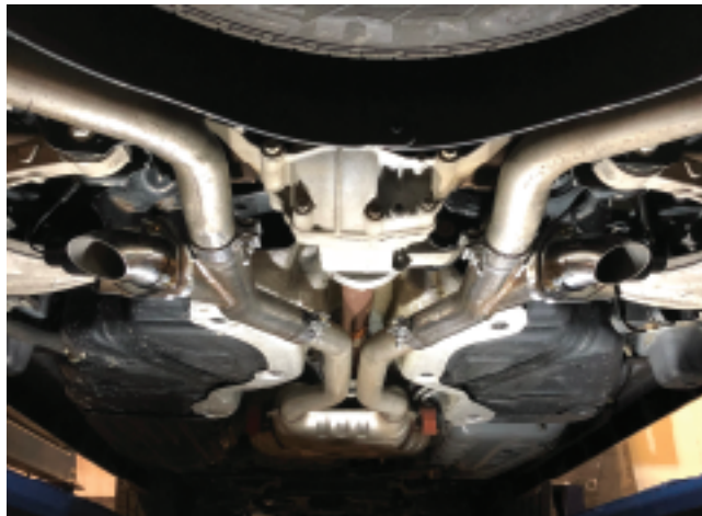
Image E: Valves and Turndowns installed viewed from rear Note motor housing location on install.
