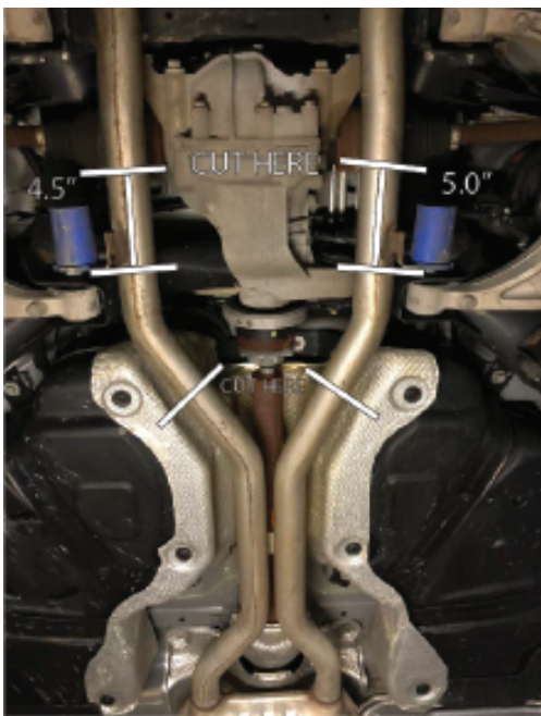
Image A: Cut Locations, measure rear cut, hold up and trace front cut.
