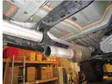
Image C: After the cut remove the resonator and De-Burr the cut.
