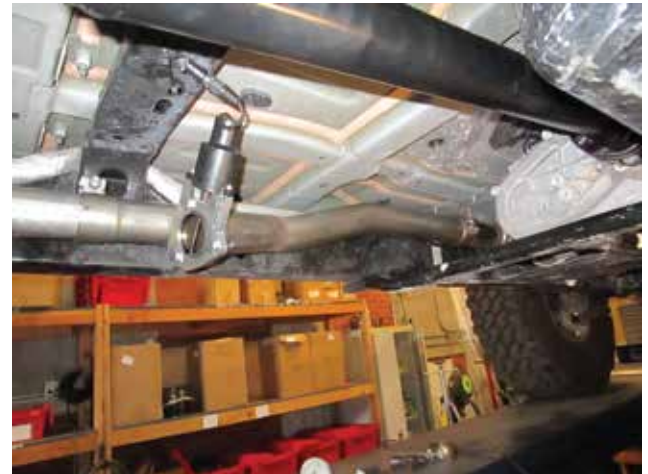
Image D: Install slipover first then the swivel seal end. orientate the valve as shown when installed.
