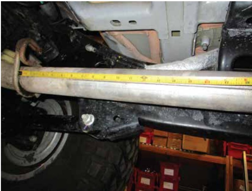
Image A: Measure from the hanger 17" towards the front of the vehicle, mark and cut the factory exhaust there.
